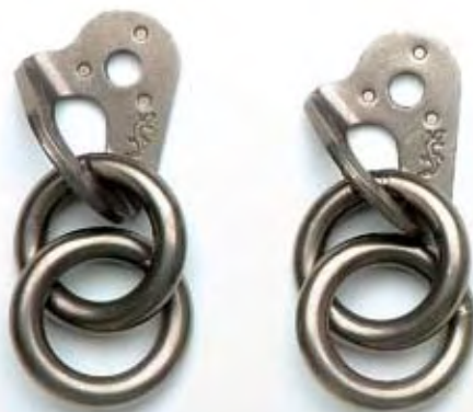
Hanger Fixe 3 Bi-chrome plated steel. Weight: 257 g. Strength: 25 kN.
